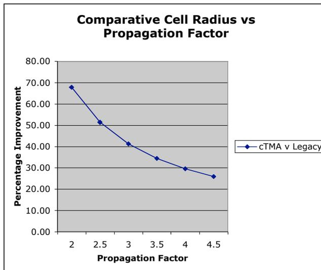
Fig. 2: **cTMA** Cell Radius Improvement vs  $\gamma$
